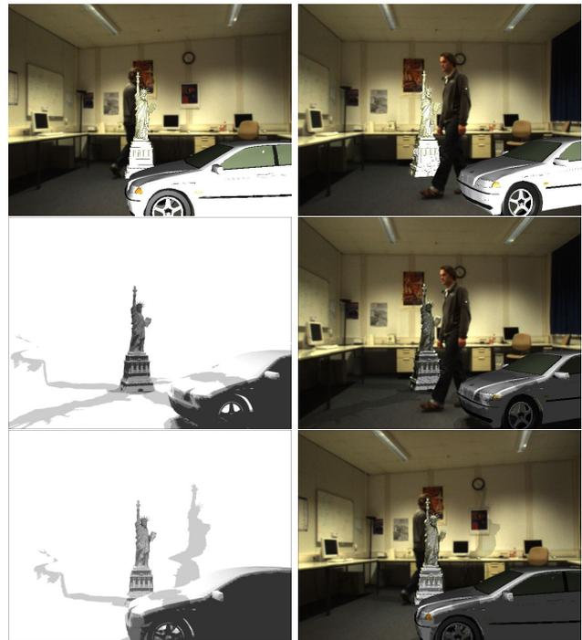
Figure 8: Top row: Mixed images without shadow computation, Middle row: Light map and image with shadows computed from light sources at the ceiling, taken from the background model. Bottom row: Light map and image with altered light source positions.
