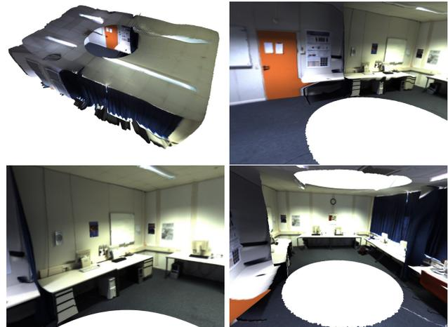
Figure 6: Full 360° reconstruction of the environment. Top Left: View of complete environment model. Others: Different views of the interior.
