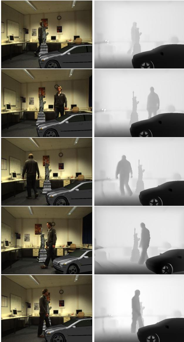
Figure 13: The final mixing result with the augmentation of virtual objects in the target camera, occlusion handling and shadow rendering.
