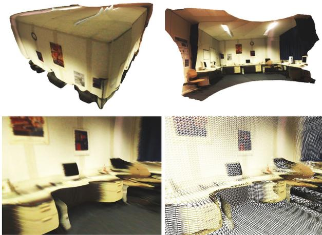
Figure 5: 3d-model of the scene corresponding to the panorama depicted in figure 4.
