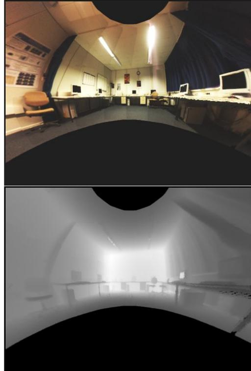
Figure 4: Cylindrical colour and depth image of the scanned panorama.
