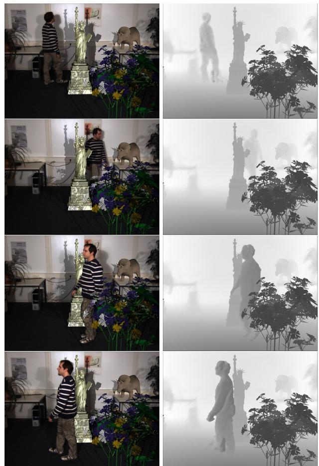
Figure 14: Final mixing result with shadow mapping. In this example two light sources are placed left and right of the camera. The real light sources have been simulated in the shadow mapping and shadow casting between virtual content and real dynamic content is visible. (Note the shadow on the legs of the person.)
