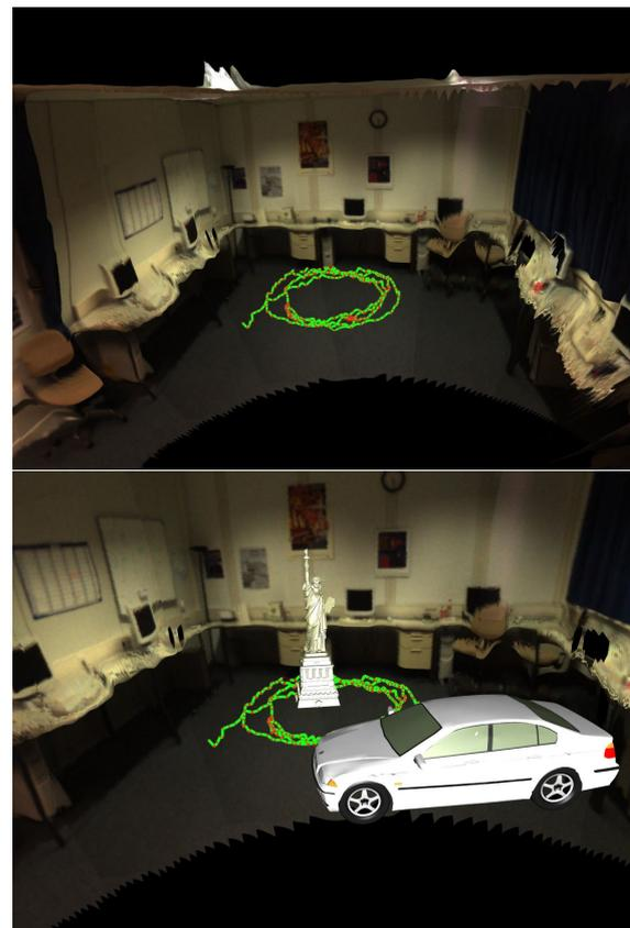
Figure 11: Top: Trajectory of the moving person projected to the ground plane. Points show the positions, connections the path of the person. Bottom: Background model with path and aligned virtual models.
