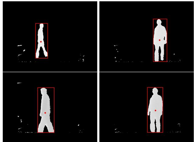
Figure 10: Tracking of dynamic content. The moving person is detected and marked with a rectangle, the center-of-mass is marked with a dot.
