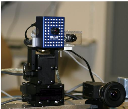
Figure 1: The used setup comprising of a ToF-camera (SwissRanger 3000) mounted together with a CCD firewire camera on a pan-tilt-unit and a fisheye camera mounted at the bottom right.
