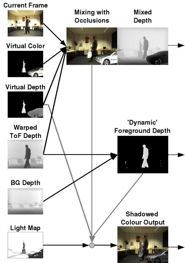
Figure 9: Overview of the mixing and shadowing done on the GPU. On the left hand side all the input images are displayed. Based on the different depth images mutual occlusions can be handled in the augmentation. Moreover foreground segmented depth images and mixed depth images are delivered. The scaling of the augmented image via the light map yields the final colour image output.
