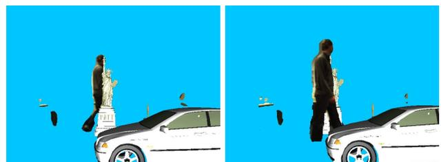
Figure 12: Mixing of real and virtually added data. In order to make the consequences of motion blur in the depth images more visible the background has been removed by depth-keying.
