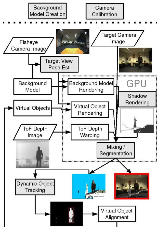
Figure 2: System components and interactions. The grey boxes are discussed in detail in the text.
