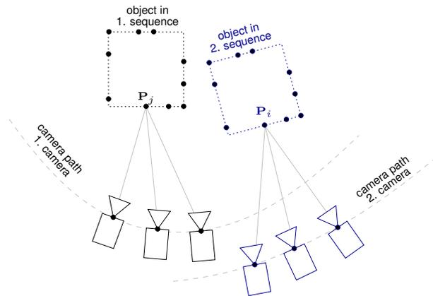
Figure 6: Registration of multiple moving cameras that capture the same scene simultaneously. Drift removal and registration of multiple cameras are similar problems, which becomes obvious, when this figure is compared with Fig. 2.
