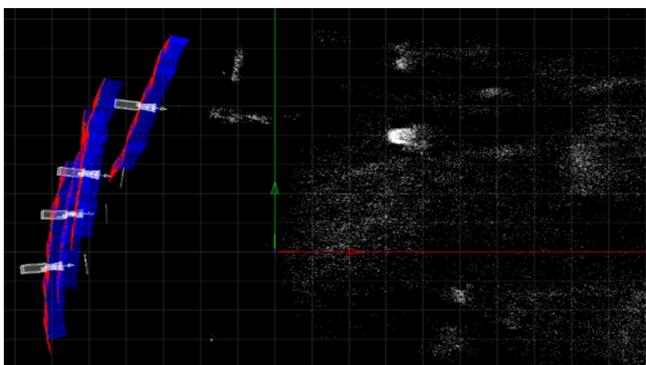
Figure 10: Top view on the resulting camera path of four moving cameras. The four independent reconstructions were registered into a common global coordinate system.
