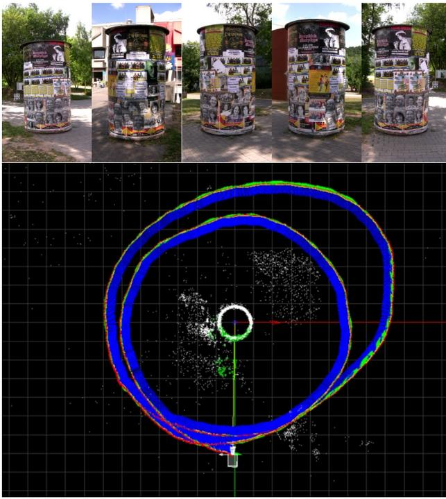
Figure 7: Five images out of the input video of example 1 and a top view on the resulting camera path after sequential structure-from-motion.
