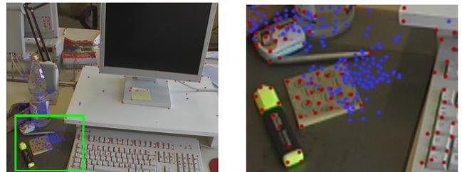
Figure 3: A real-world example of drift. After the camera revisits the same part of the scene the 3D object points of the current image (red) differ strongly from the 3D object points generated earlier in the sequence (blue). The right image shows a detail magnification from the left image. The squared shape of the yellow paper is clearly visible in the shifted blue point cloud.
