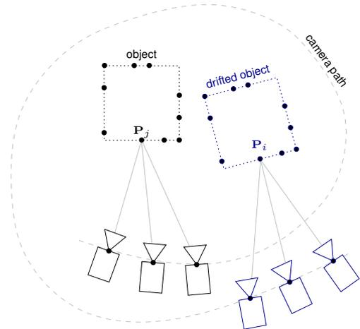
Figure 2: After processing a long sequence 3D object points  $\mathbf{P}_j$  and  $\mathbf{P}_i$  are not at the same position because of drift.
