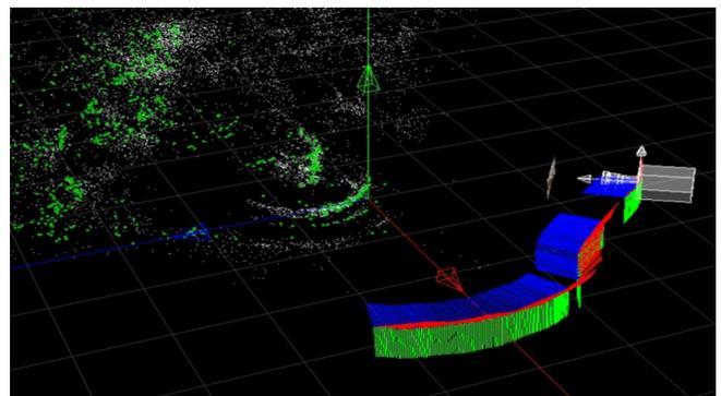
Figure 12: Camera path and 3D object point cloud after registration of three independent structure-from-motion estimations in example 3
