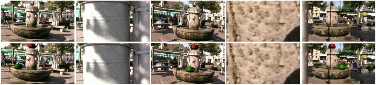
Figure 11: Top row: Five images out of the input video of example 3. The motion estimation has to restart two times because of large occlusions in the foreground. These large occlusions are visible in the second and fourth image of the top row. Bottom row: Augmented video sequence.
