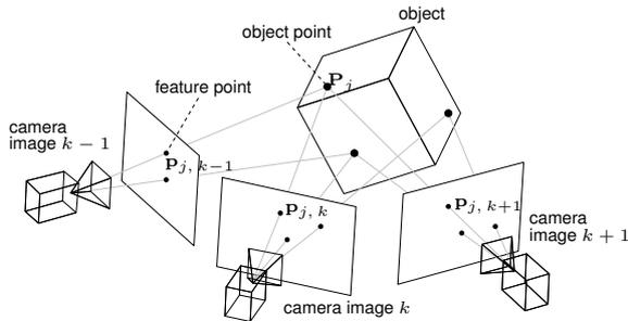
Figure 1: Result after structure-from-motion estimation. The projection of a 3D object point  $\mathbf{P}_j$  in the camera image at time  $k$  gives the tracked 2D feature point  $\mathbf{p}_{j,k}$ .
