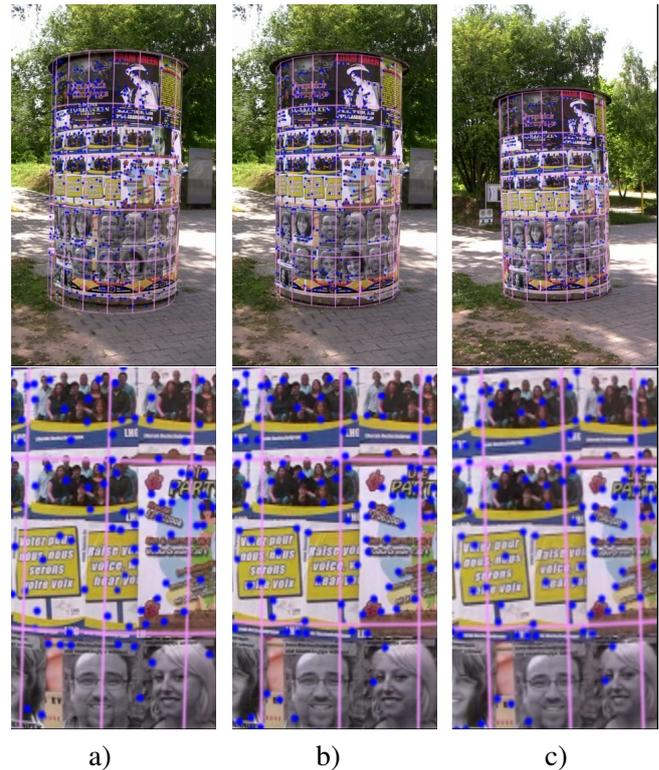
Figure 8: a) result without drift removal after two loops around the column, b) result with drift removal, c) first frame of the sequence as drift-free reference. Only the 3D object points that were generated in the first frame are shown as blue dots. The second row shows detail magnifications of the above images.
