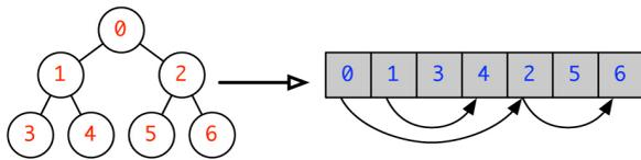
Figure 4: Depth-first left ordered binary tree serialization.
