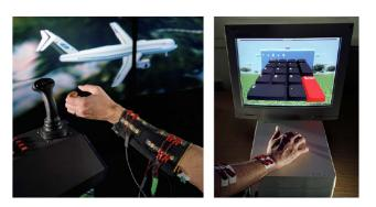
Figure 1: EMG Arm Joystick [WJ03]
