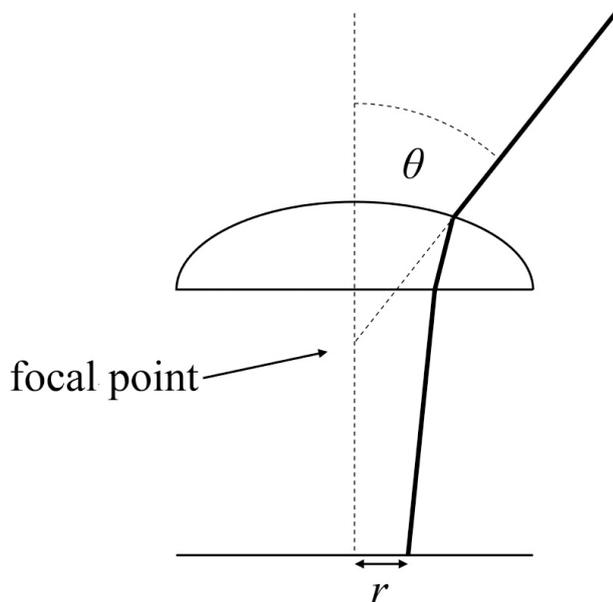
Figure 3:  $\theta$  and  $r$  in a fisheye lens
