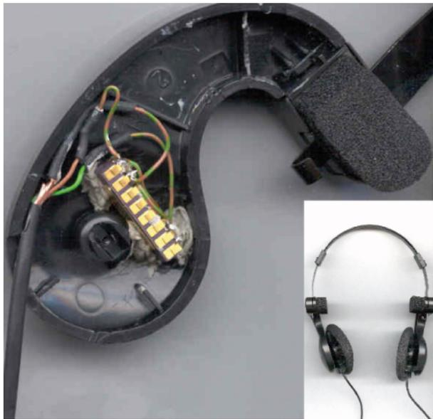
Figure 3: The sensor was integrated into a Koss headphone and (later) clad with casting resin.
