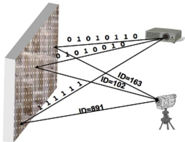
Figure 2: Active registration using binary coded point patterns.
