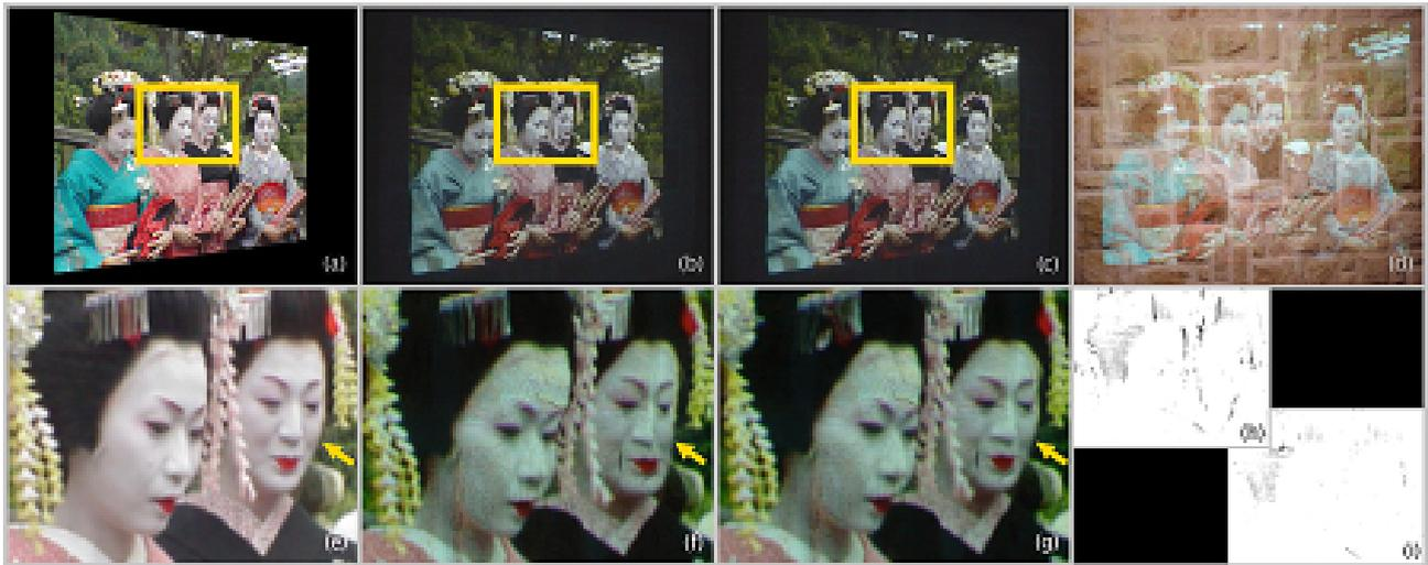
Figure 5: Passive calibration results: ideal image (a) and close-up (e), uncorrected image (b) and close-up (f), corrected image (c) and close-up (g), image without radiometric compensation under environment light (d), visualized error maps for uncorrected (h) and corrected (i) case.
