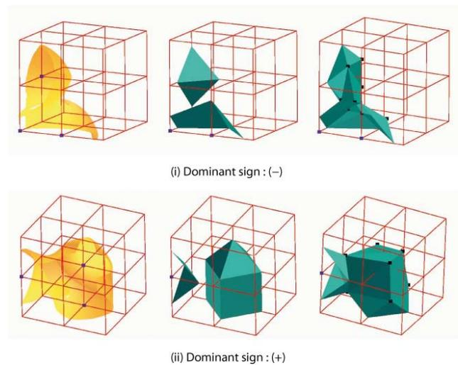
Figure 10: Trilinear surface (left), MC result (middle), and Dual Isosurfacing result (right) for 2x2x2 synthetic dataset with a tunnel and one ambiguous face.
