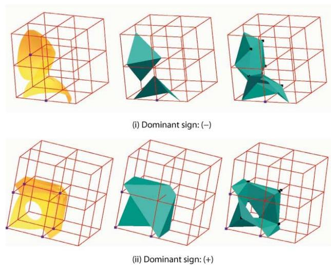
Figure 9: Trilinear surface (left), MC result (middle), and Dual Isosurfacing result (right) for 2x2x2 synthetic dataset with a tunnel and no ambiguous faces.
