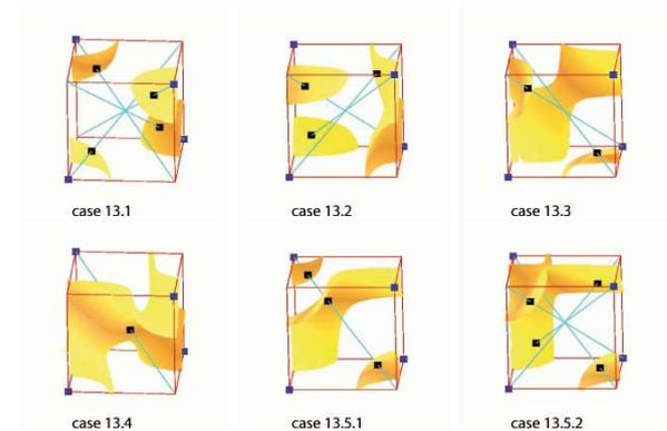
Figure 7: Topological configurations with six ambiguous faces: trilinear model in yellow-orange, isopoints in black, positive nodes in blue, rays in cyan.
