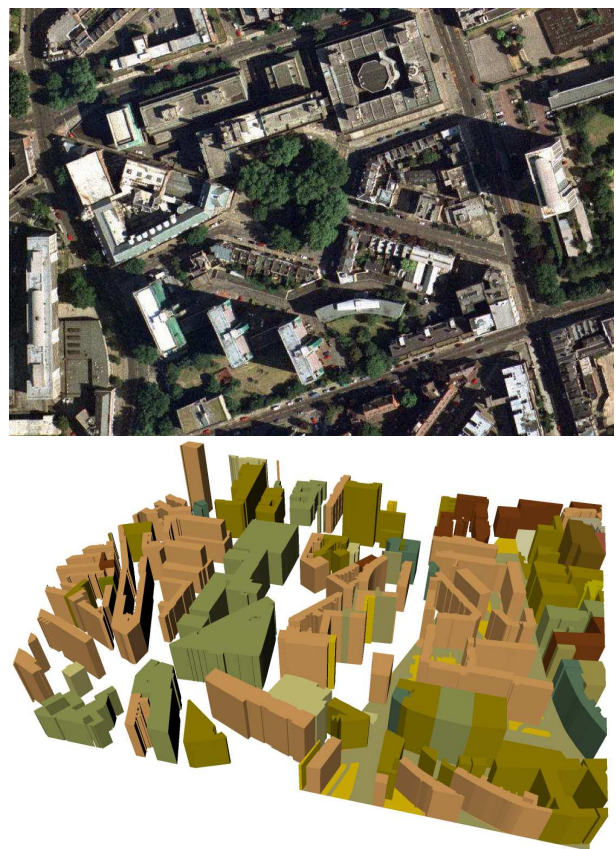
Figure 1: Accurate modelling of urban environment (a) high resolution aerial image (b) 3D building extruding
