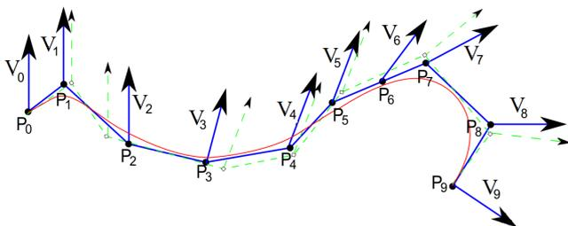
Figure 13: Green line connects initial position points, green dashed vectors are initial orientation vectors, red line is a B-spline position curve, blue line is the control polygon of B-spline position curve with control points  $P_0, \dots, P_9$ , blue vectors  $V_0, \dots, V_9$  are generated new orientation vectors starting from position control points.
