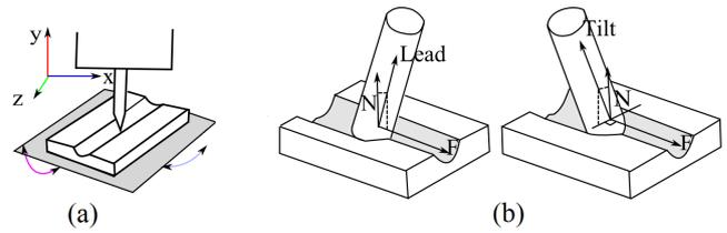
Figure 1: (a) 5-axis machining. (b) Orientational information of the tool in form of lead and tilt
