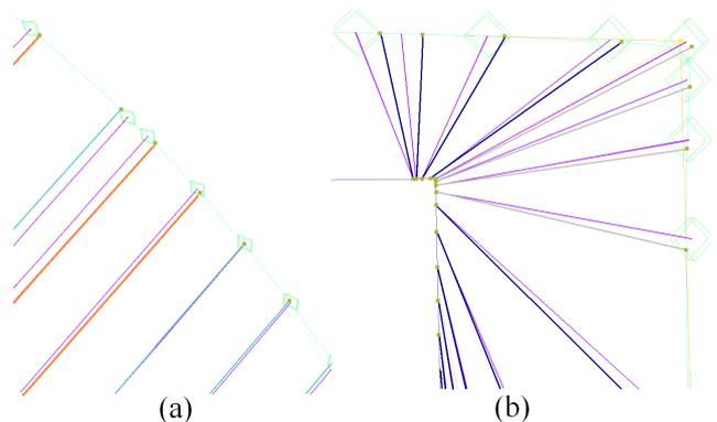
Figure 29: Parts of the workpiece. Purple lines are interpolated orientation vectors. (a) Zoomed-in rounded part, see Figure 28a. Orange lines are resulting vectors with delay, light blue are resulting vectors with overdrive. (b) View of the turn from the top, see Figure 28b. Gray and dark purple lines are resulting vectors on opposite sides of the polygon.
