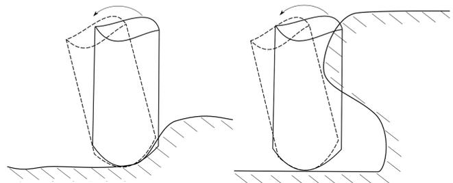
Figure 3: Gouging (left) and collision (right).
