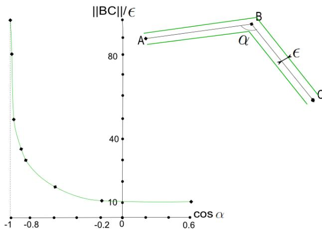
Figure 9: Point insertion criteria. If the distance divided by the tolerance of the channel is above the curve, then we insert the point in the middle between initial points B and C.
