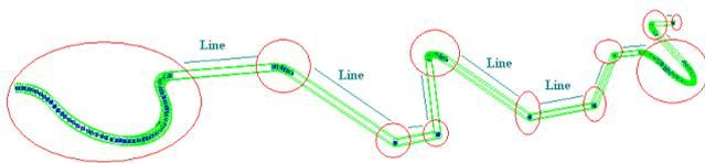
Figure 7: Line connections between groups of points that are further apart than distance  $d_{max}$ . Dots represent control points, which form groups encircled in red that are connected by straight lines.
