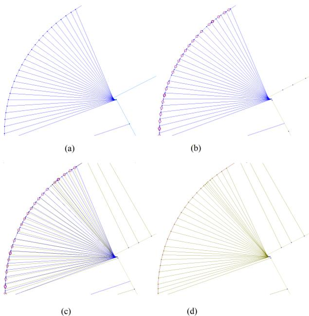
Figure 21: Outline of the process of generating a 5-axis tool path optimization for a 90° turn. (a) Initial position and orientation data. (b) Constructed frustums. (c) Generated orientation vectors and curve. (d) Resulting B-spline curves.
