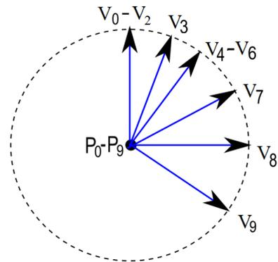
Figure 14: Described algorithms use the sphere representation to solve the orientation part of the problem. Generated orientation vectors  $V_0, \dots, V_9$  from the Fig. 13 are placed at the origin of a sphere such that control points  $P_0, \dots, P_9$  coincide. We can see that  $V_0, V_1$  and  $V_2$  are the same for this example, because they have the same directions in Fig. 13.
