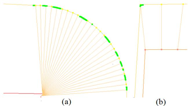
Figure 23: Parts of the workpiece. High curvature (higher than one) of the orientation curve are highlighted by green points, red line is a position B-spline curve, orange lines are orientation vectors and orientation polygon. (a) Rounded parts. (b) Turns.
