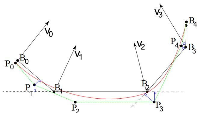
Figure 10: Control points determination to a proper interval. Arrows  $V_0, \dots, V_4$  indicate initial orientation vectors, where the starting points of these vectors are the initial position points  $B_0, \dots, B_4$ .  $P_0, \dots, P_4$  are optimized control points of the local position B-spline curve (red curve), blue lines are perpendiculars to lines formed by  $B_0, \dots, B_4$ .
