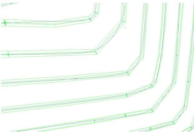
Figure 18: Smooth curve (blue) within tolerance channel (green) at sharp corners.
