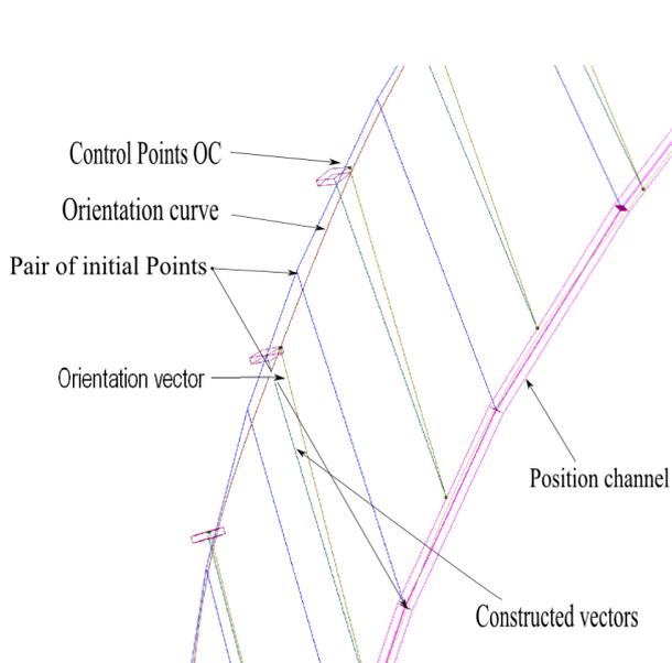
Figure 20: Optimized 5-axis tool path.
