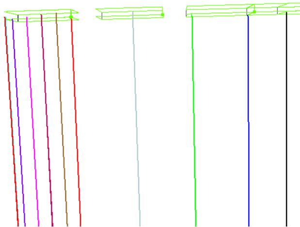
Figure 26: Resulting vectors and its frustums for the problem transformed into the sphere problem. All orientation vectors (lines of different color) start from one position, which is the center of the sphere.
