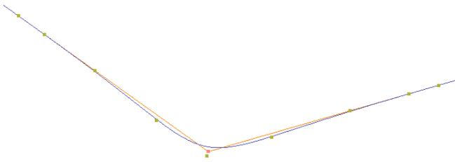
Figure 6: Symmetric solution for a single corner point, where the red curve is the control polygon and the blue curve is the solution.
