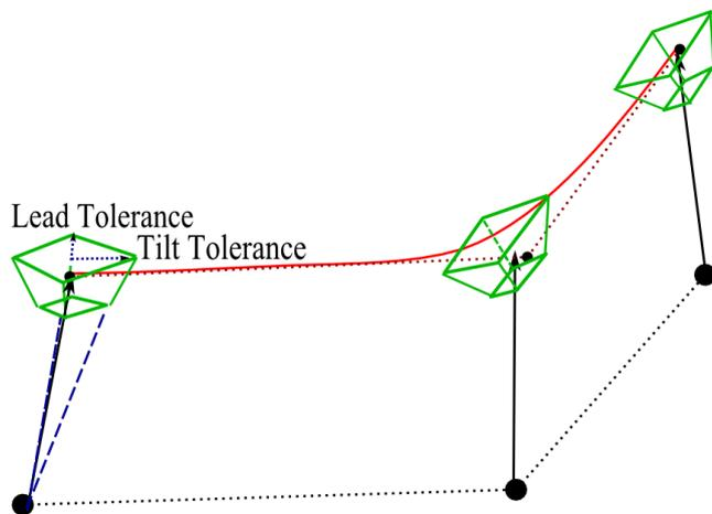
Figure 2: Black vectors are newly generated orientation vectors starting from the optimized position control points. Frustums (green) are built with respect to given tolerances for lead and tilt (blue). Red curve is the resulting B-spline orientation curve with the control polygon shown as dotted dark-red lines.
