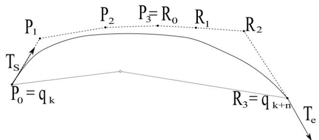
Figure 12: Local non-rational cubic curve approximation
