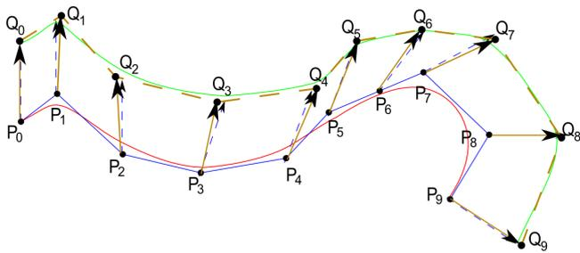
Figure 16: Obtained solution on the sphere is transformed back to the initial problem using formula  $Q_i = P_i + Q'_i$ . Brown vectors are the final orientation of the tool, red line is a position B-spline curve, green line is an orientation B-spline curve, dashed brown line is a control polygon of orientation curve. The two B-spline curves have the same knot vector.
