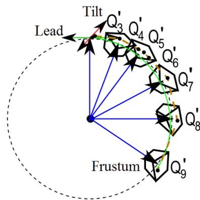
Figure 15: Frustums are built around every vector to restrict control points  $Q'_i$  to lie inside these frustums. Control Points  $Q'_4, Q'_5, Q'_6$  lie inside matching frustums formed around collinear vectors  $V_4, V_5, V_6$  but they do not need to be placed at the same position. Brown dashed line is a control polygon  $Q'_0, \dots, Q'_9$  of the green B-spline curve.
