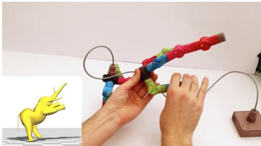
Figure 4: Modular tangible input device for character animation (from [JPG<sup>+</sup>14]). With its embedded sensors, this physical prop is used to precisely drive a virtual object.
