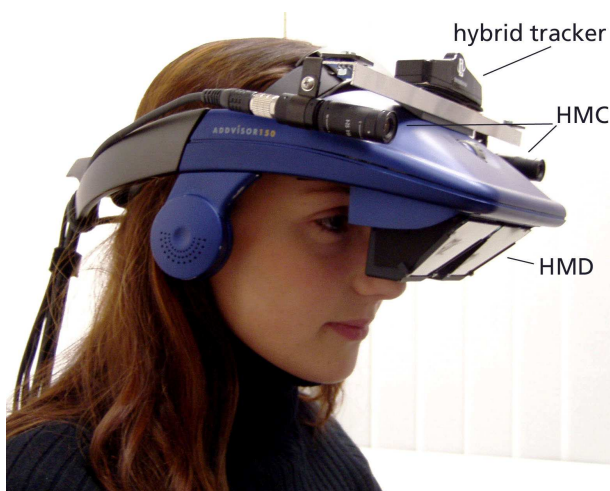
Figure 2: ARTHUR See-through head mounted display (HMD).
