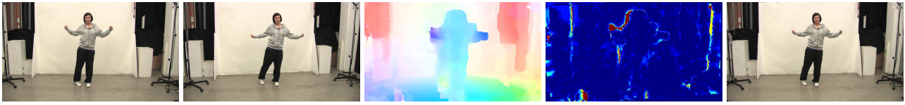
Figure 1: Belief Propagation Optical Flow. Left to right: two 1920 \times 1080 input images A and B , optical flow from A to B , flow symmetry, rendered in-between image. We specifically tailored our optical flow for image morphing in the presence of large motion and occlusions. We incorporate recent advances in computer vision to produce visually convincing results.
