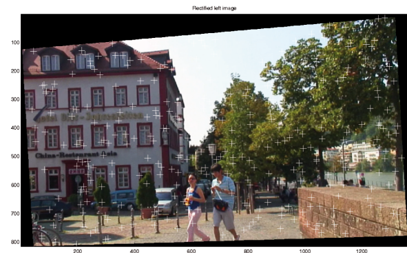
Figure 5: Quasi-Euclidean stereo image rectification [FI08] using a randomly sampled subset of correspondences. For visualization purposes, only 300 out of the 10,000 sampled correspondences are rendered on top of the rectified image.
