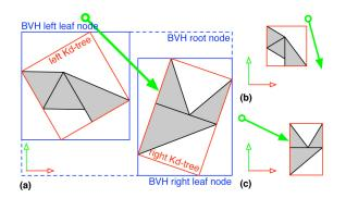
Figure 5: Detailed schematic view of the TLH traversal. Figure (a) Shows the top-level BVH within the global coordinate system. During TLH traversal the ray intersects both BVH child nodes therefore it has to be transformed to both local Kd-tree coordinate systems. Figures (b) and (c) show the traversal of the Kdtrees in their local coordinate space.
