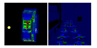
Figure 8: These images illustrate the amount of Kdtree traversals for the first shadow ray traversal for the chevy scene and the BART robots scene. Blue colors indicate up to three, green colors up to six, red colors up to nine and white color more than nine Kd-tree traversals per ray.
