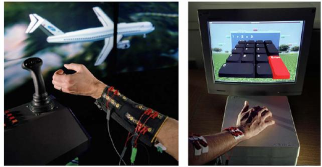
Figure 1: EMG Arm Joystick [WJ03]
