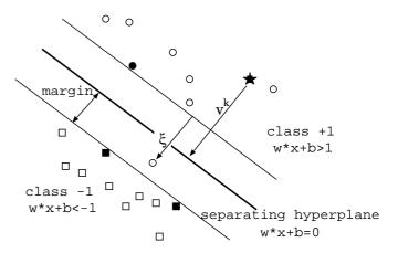
Figure 2: **Operating mode of a Support Vector Machine.** The SVM algorithm seeks to maximise the margin around a hyperplane that separates a positive class (marked by circles) from a negative class (marked by squares).
