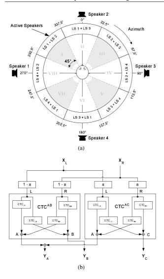
Figure 8: Partitioning into sectors and dynamic 3channel CTC filter structure with cross-fade.
