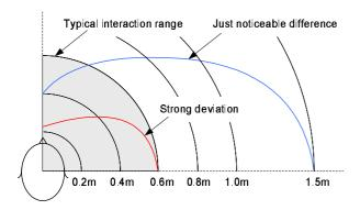
Figure 6: Limits of noticeable differences between near-field and far-field HRTFs. The gray area marks the typical interaction range in a room-mounted VR CAVE-like display.
