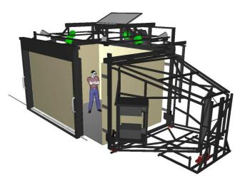
Figure 3: Five sided projection CAVE-like virtual environment using optical tracking. Possible loudspeakers are colored in green and mounted on the rack on top of the device.
