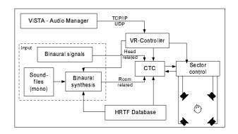
Figure 9: Complete system for virtual acoustical imaging.
