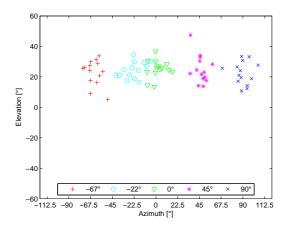
(a) Localization results for sources at 30 degree elevation
