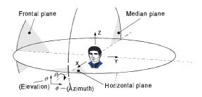
Figure 5: Specified frame of reference for head movements and rotations.
