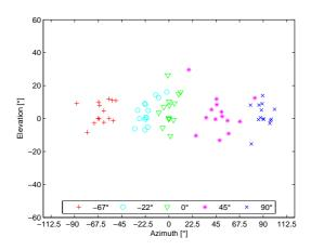
(b) Localization results for sources at 0 degree elevation
