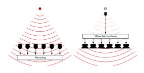
Figure 2: Setup for recording a sound field and reproducing it by wave field synthesis.
