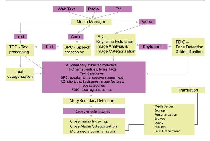
Figure 3: The REVEAL THIS system architecture
