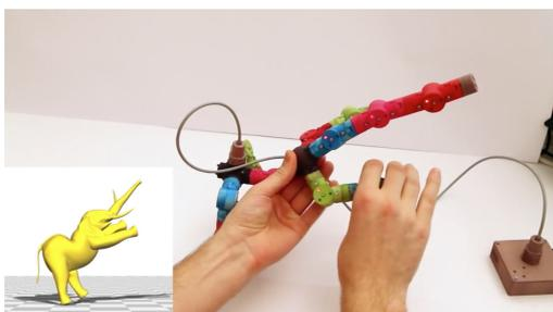
Figure 4: Modular tangible input device for character animation (from [JPG<sup>+</sup>14]). With its embedded sensors, this physical prop is used to precisely drive a virtual object.
