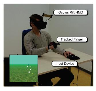
Figure 4: User during the experiment. The inset shows the user's view to the VE with the white and blue target spheres as well as the yellow sphere that visually represents the tracked finger tip.
