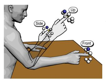
Figure 5: Schematic illustration depicting the three interaction positions. Only one ring of spheres was active during a single trial. The blue sphere depicts the target sphere. The yellow sphere depicts the sphere the user saw at the location of the fingertip.
