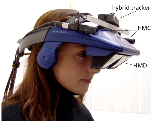
Figure 2: ARTHUR See-through head mounted display (HMD).
