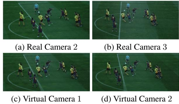
Figure 12: Synthesis of the virtual images at frame 50. The color information of the real cameras (a-b) is transferred into two virtual cameras (c-d).
