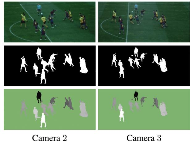
Figure 8: Depth estimation at frame 50. The original images are presented in the first row for the central real cameras 2 and 3. The corresponding segmentations and the depth estimations are then shown in the second and third rows. The depth colors correspond to the depth planes: the lighter color, the closer to the cameras.
