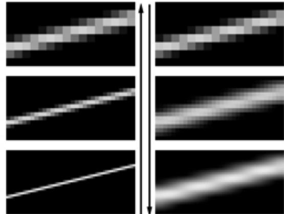
Figure 9: Pyramidal blurring of an antialiased line with the biquadratic analysis filter.
