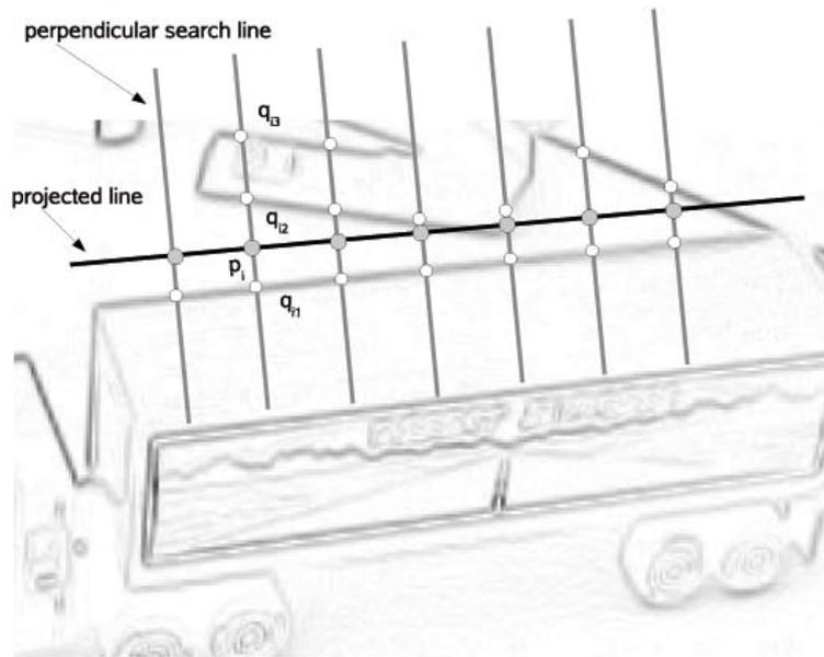
Figure 2: Perpendicular search for gradient maxima.  $p_i$  is a point on the projected 3d line.  $q_{ij}$  are hypotheses of the corresponding points in the image.
