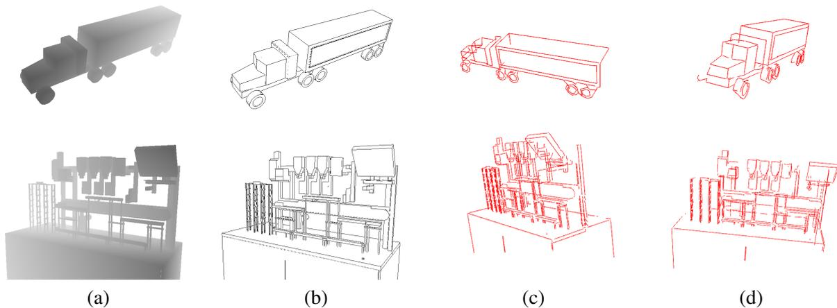
Figure 1: 3D Line extraction using discrepancies in the z-buffer. (a) shows a z-buffer image. (b) illustrates an edge image obtained by a Laplacian Filter. (c) and (d) show the generated 3D line model of different views.
