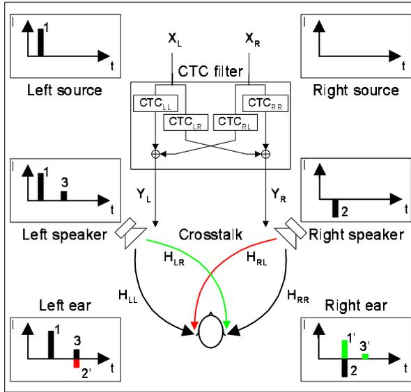
Figure 7: Principle of static crosstalk cancellation. Presenting an impulse addressed to the left ear (1) and the first steps of compensation (2, 3).
