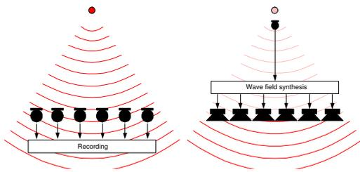
Figure 2: Setup for recording a sound field and reproducing it by wave field synthesis.
