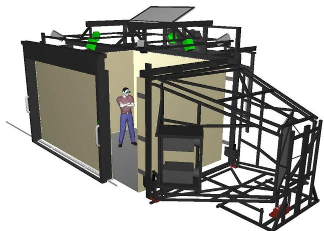
Figure 3: Five sided projection CAVE-like virtual environment using optical tracking. Possible loudspeakers are colored in green and mounted on the rack on top of the device.
