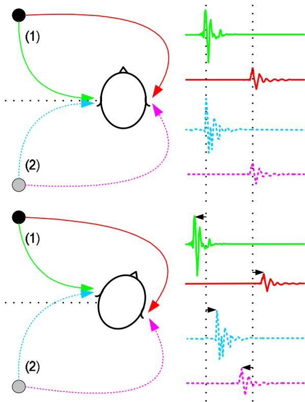
Figure 4: Variance of ITD depending on the relative head orientation of the user.
