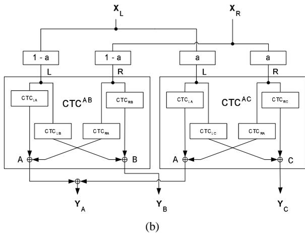
Figure 8: Partitioning into sectors and dynamic 3-channel CTC filter structure with cross-fade.
