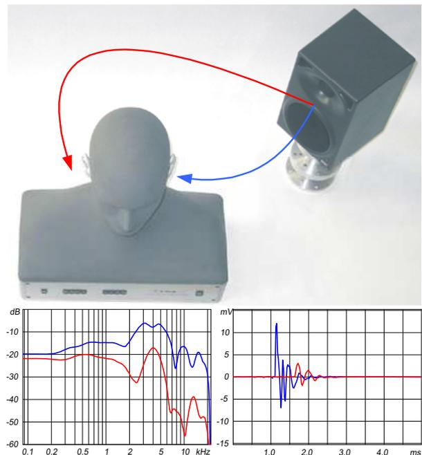
Figure 1: HRTF (smoothed with 1/6 octave bandwidth) and HRIR of a sound source under 120 degree measured using the artificial head of the Institute of Technical Acoustics of RWTH Aachen University.
