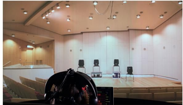
Figure 4: Optical VE (stereoscopy switched off for the photograph). In front: person with extraaural headset and tracking sensor
