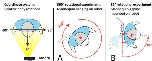
Figure 4: Drawing of coordinate system and two experimental setups: A) 360° rotation, B) 85° rotation
