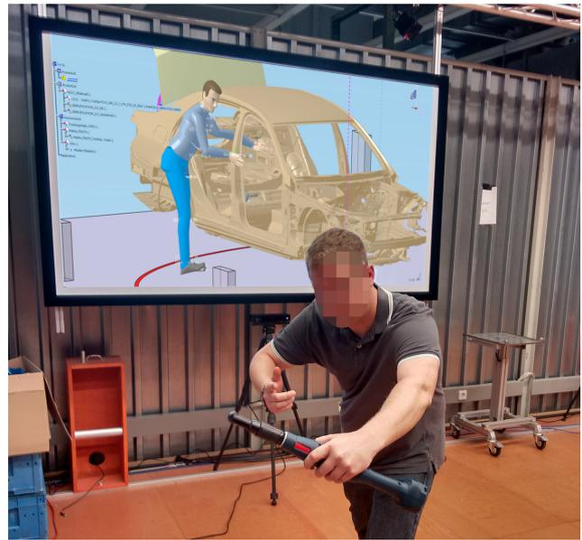
Figure 13: Delmia V5 DHM directly manipulated by marker-less motion capture approach. All assessments can be carried out in real time.
